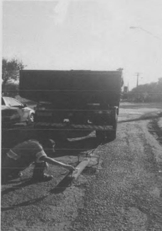
FIGURA 01: VIGA BENKELMAN
