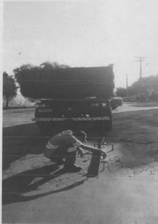
FIGURA 04: VIGA BENKELMAN
