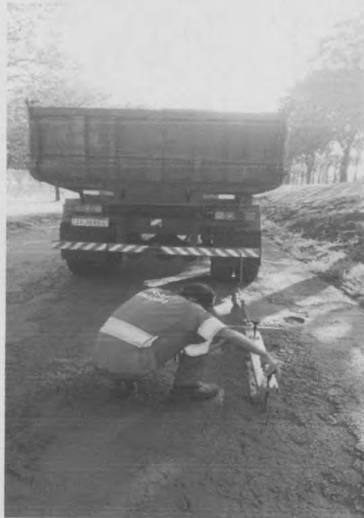
FIGURA 02: VIGA BENKELMAN
