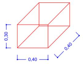
DETALHE DIMENSÕES DO BLOCO
